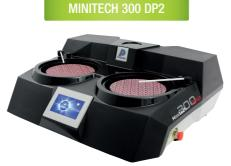
Ref. 66450 Width : 1100 mm Nb plateau(x) : 2 Depth : 810 mm Motor(s): 2 Height: 330 mm Watering ramps(s) : 2 Weight: 70 kg
